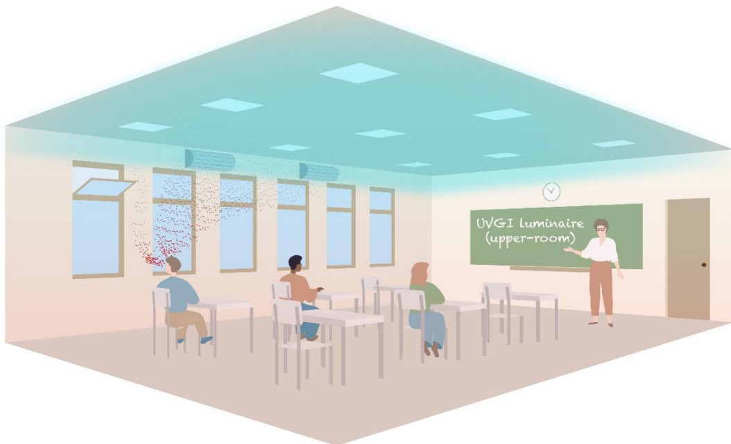
Figure 4: Illustrative example of UVGI upper-room luminaire application, combined with natural ventilation
