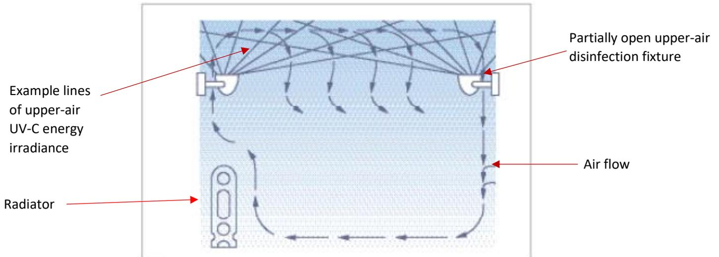
Fig 3. Graphical representation of partially open upper-air disinfection fixture space application
