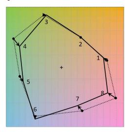
NOTE The numbers in the figure represent the TCS#, the dotted line connects the  $U^*$ ,  $V^*$  coordinates for the reference illuminant and the solid line for the test light source, where the arrows indicate the direction of the colour shifts (from the coordinates for the reference illuminant to the coordinates for the test source).
